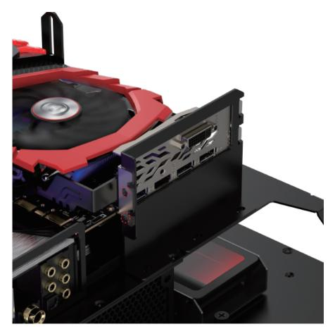
■Tighten the screws to secure the video card.
